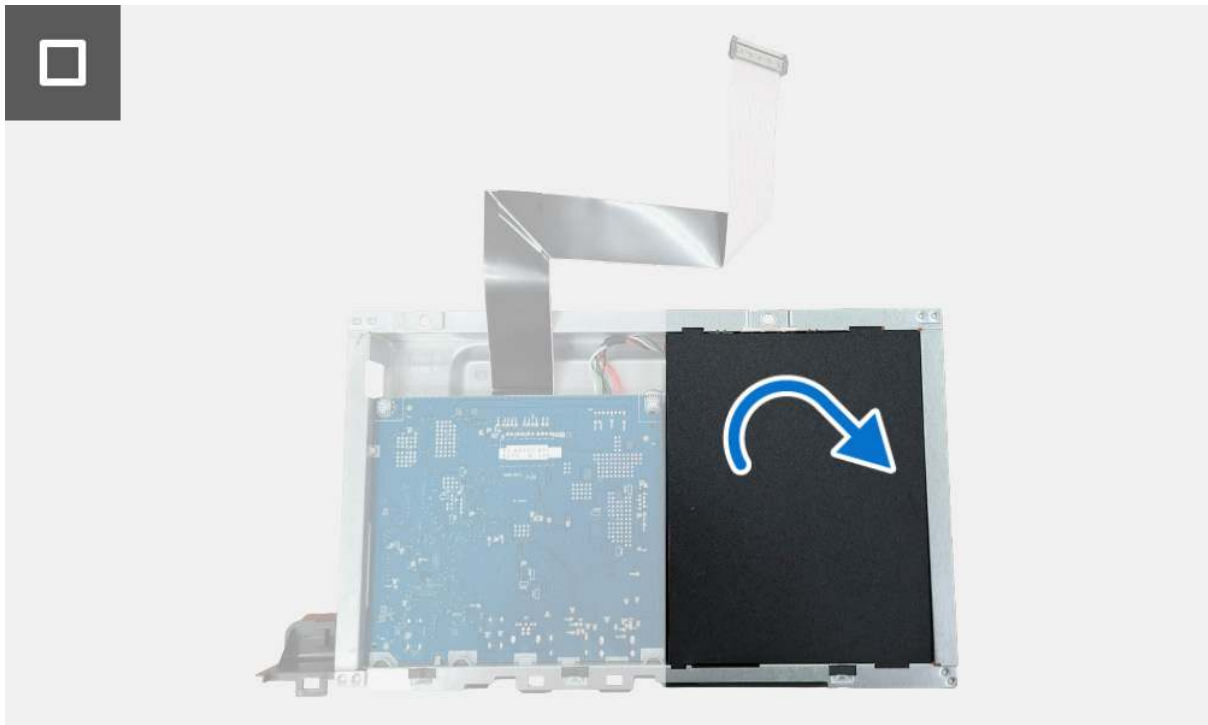
Figure 29. Installing the power board
