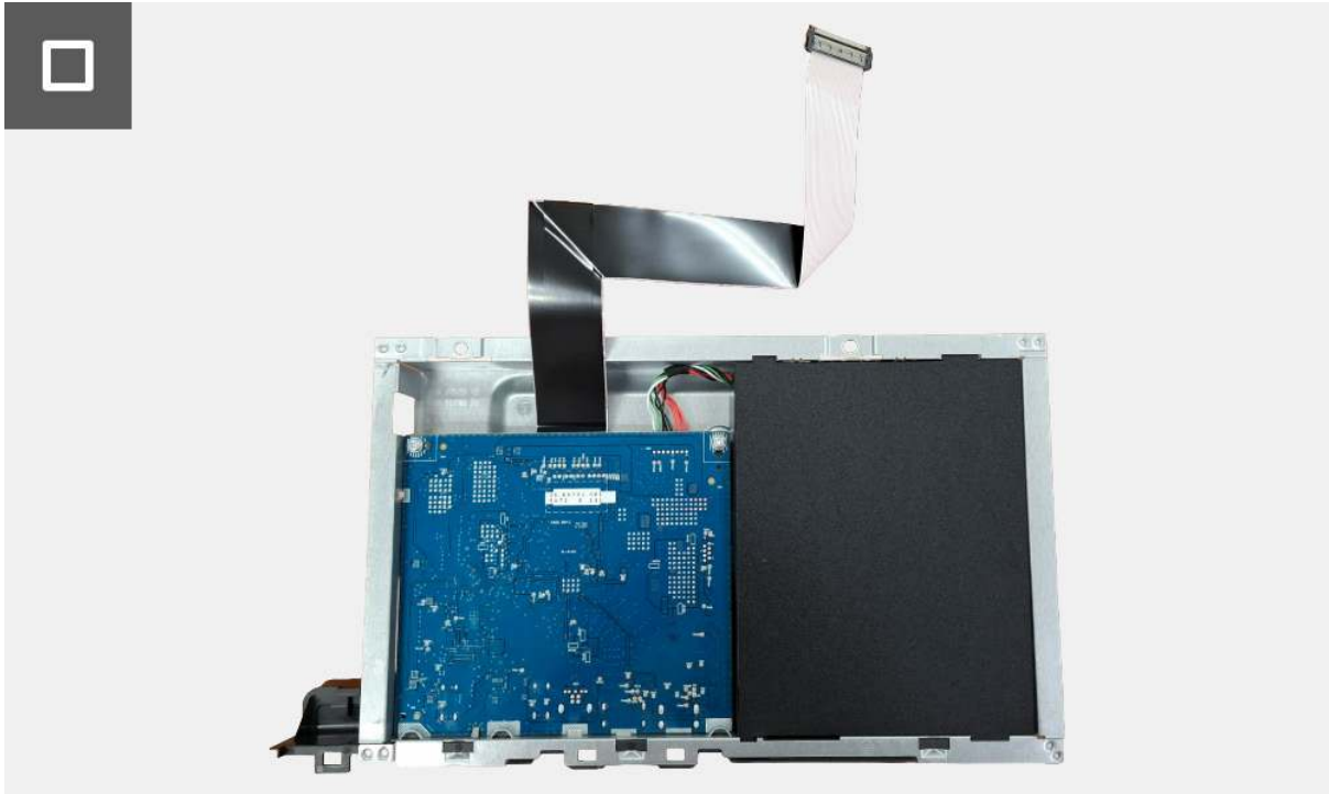
Figure 20. Removing the metal shield
