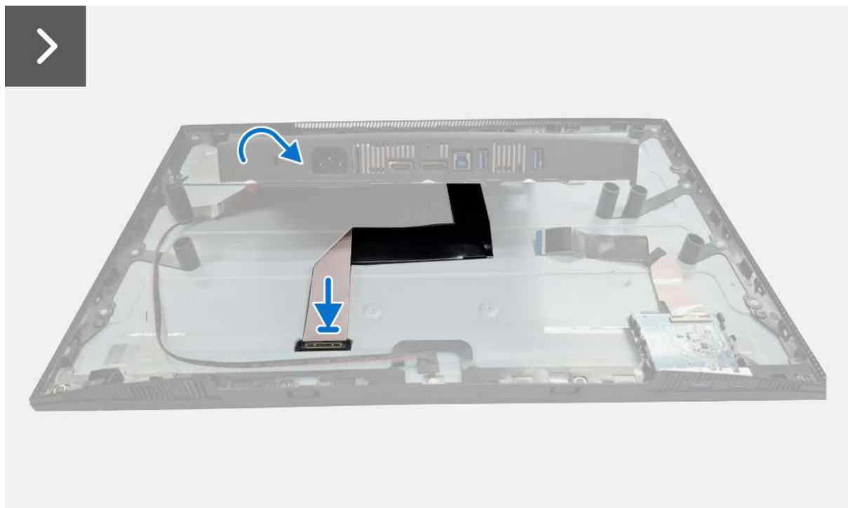
Figure 21. Installing the metal shield
