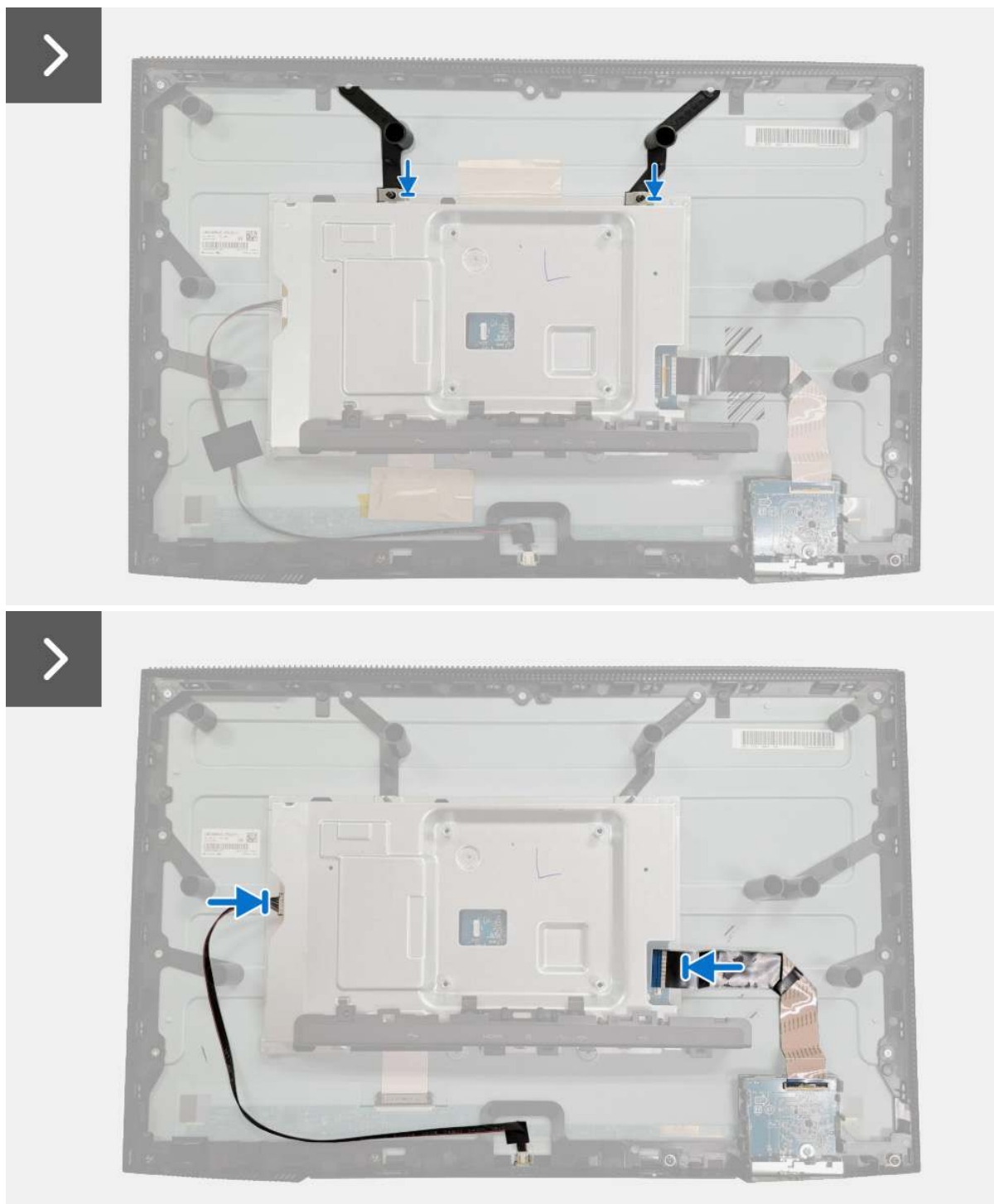
Figure 22. Installing the metal shield
