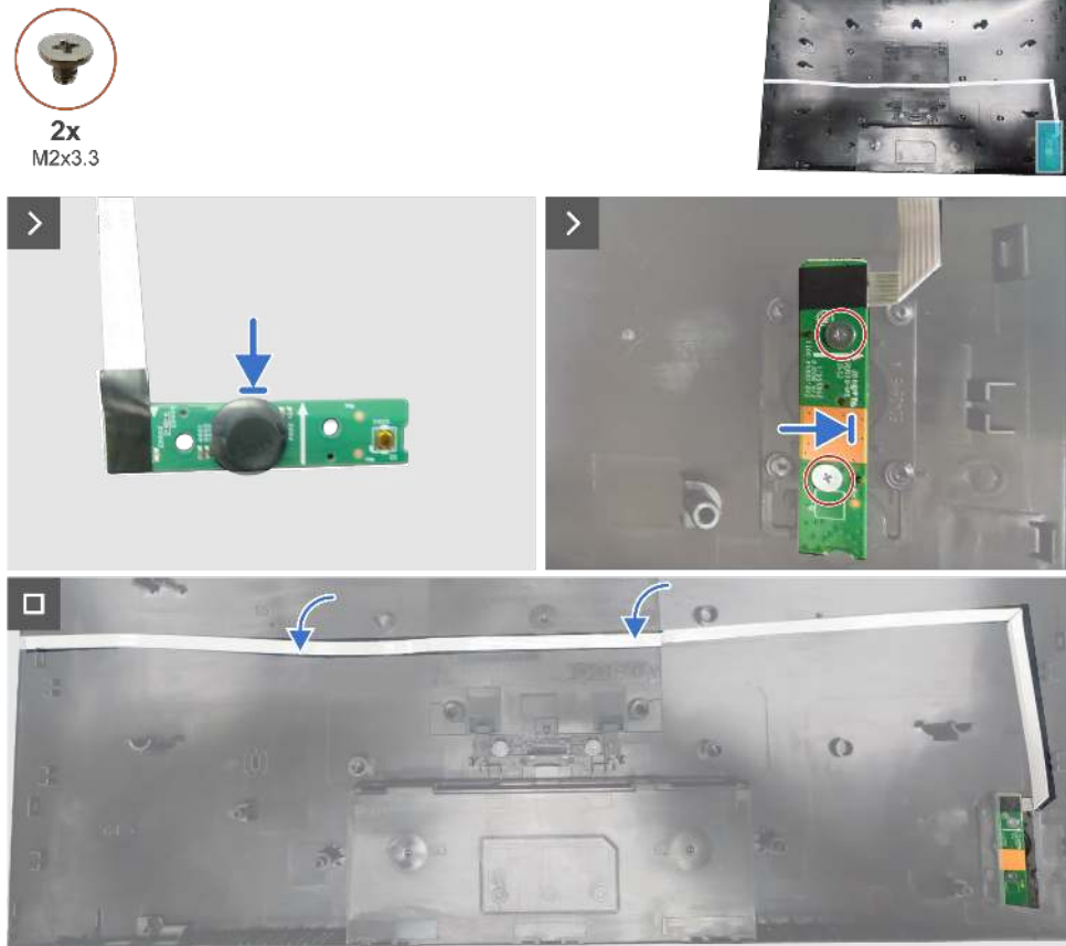
Figure 20. Installing the keypad board
