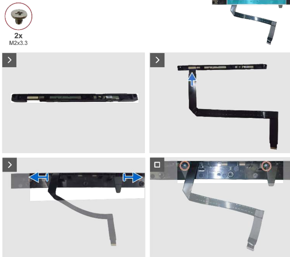
Figure 28. Installing the camera module
