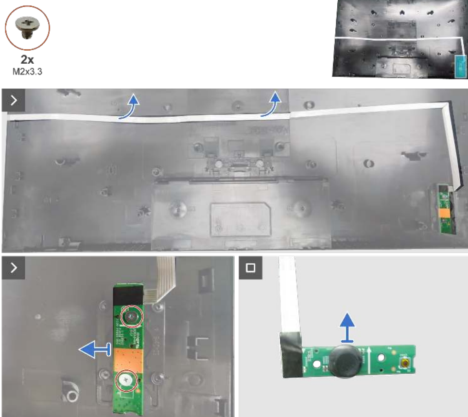
Figure 19. Removing the keypad board
