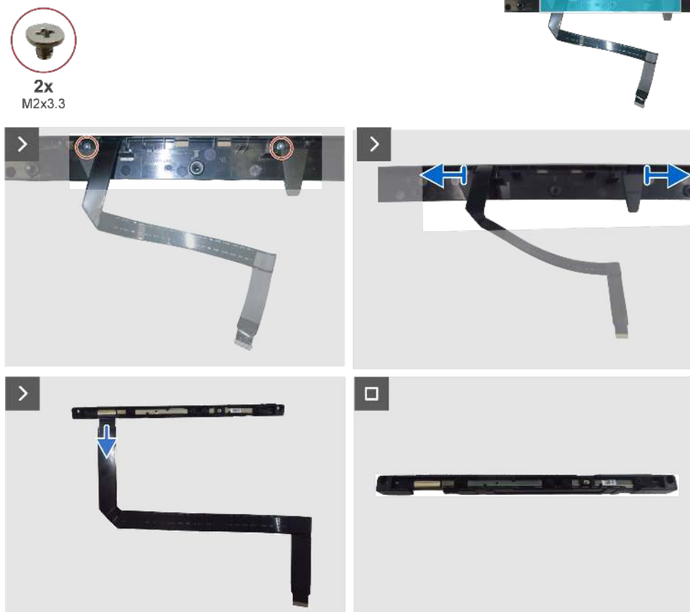
Figure 27. Removing the camera module
