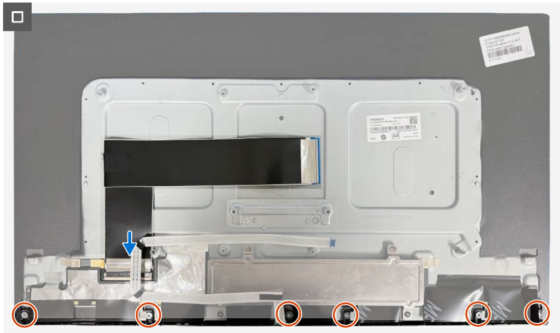
Figure 28. Installing the LED board
