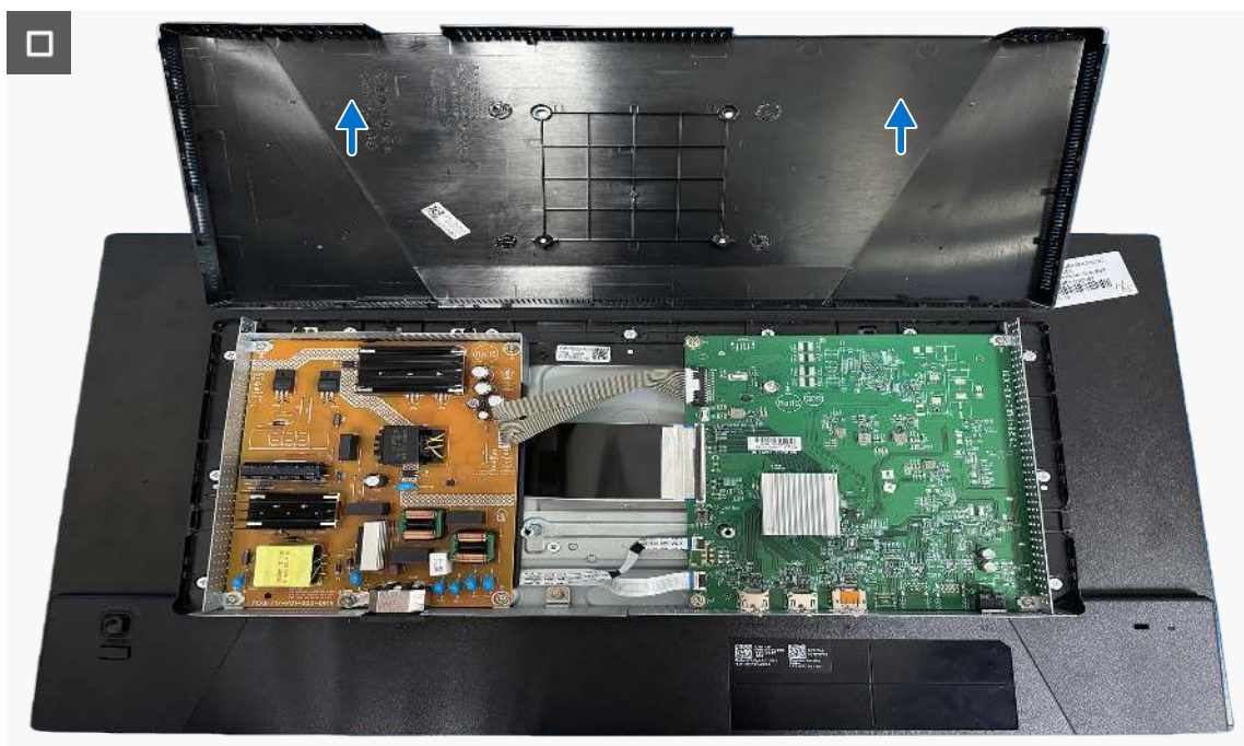
Figure 15. Removing the back cover
