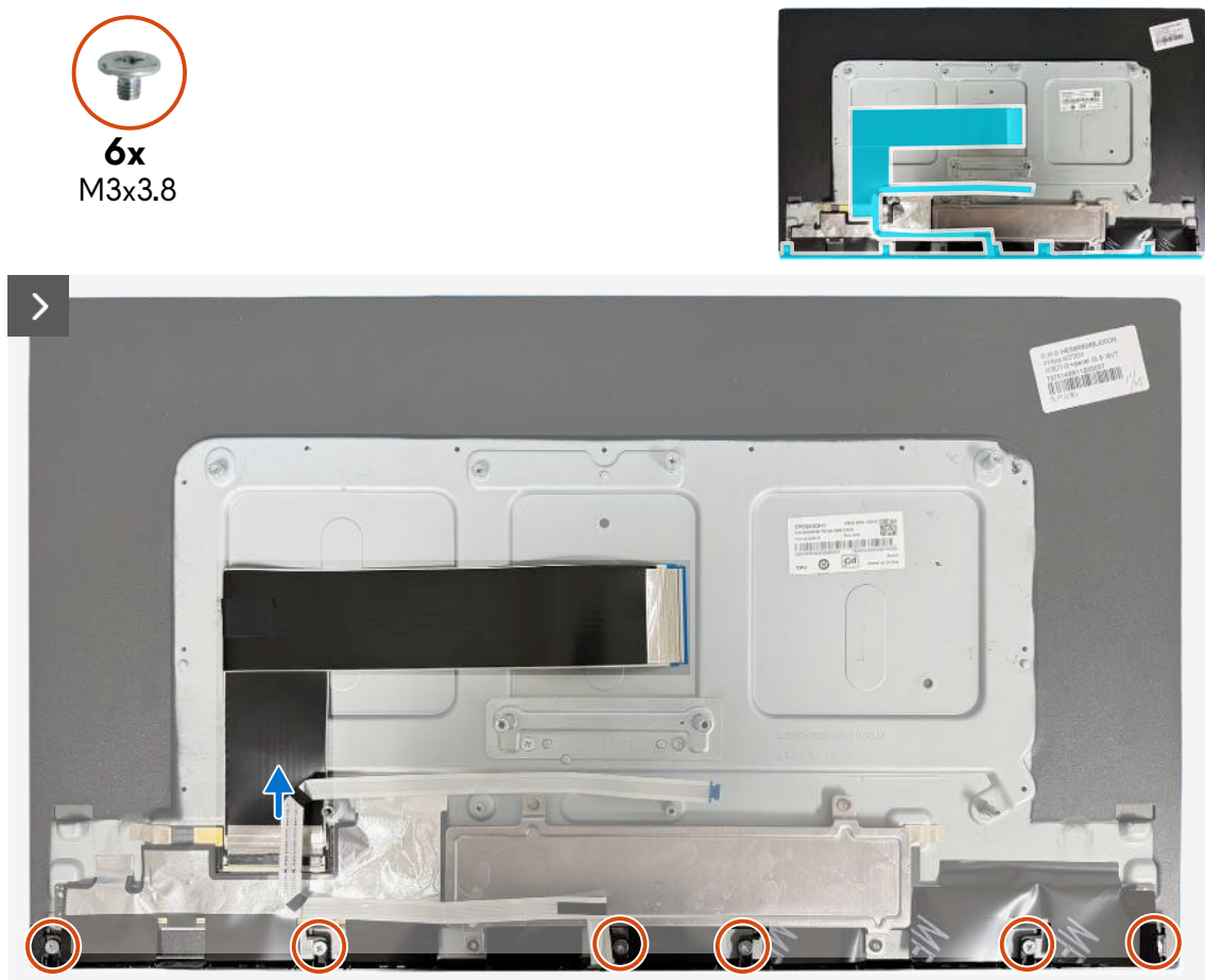
Figure 25. Removing the LED board
