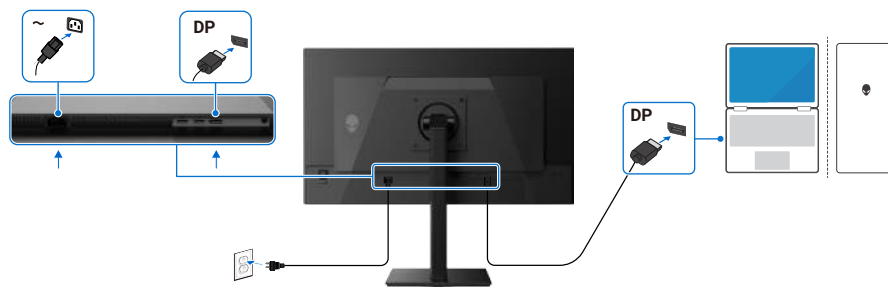
Figure 8. Connecting the DisplayPort cable
