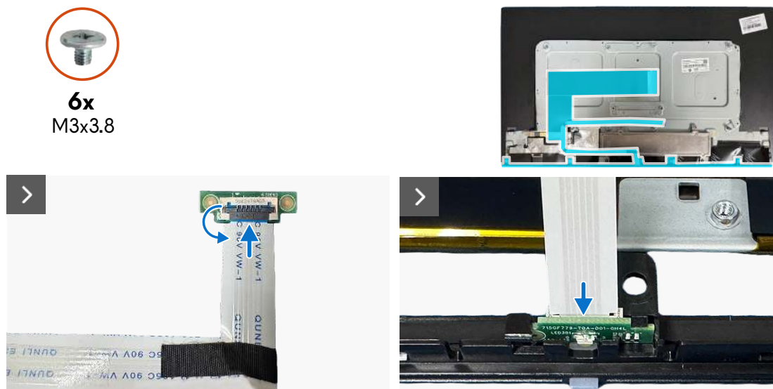
Figure 27. Installing the LED board
