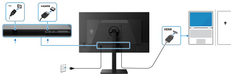
Figure 9. Connecting the HDMI cable
