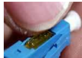
Lock the fiber inside the connector by pressing the amber button
