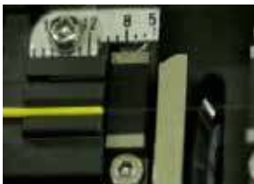
Cleave your fiber strand to 10mm from first measurement mark
