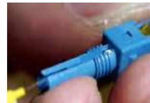
Insert the fiber into the connector body until the strand meets resistance and arches
