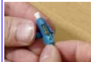
To remove or re-terminate the connector, simple unscrew the boot and replace the jig
