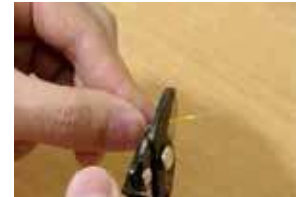
Strip 10mm of buffer using the small hole on the stripper
