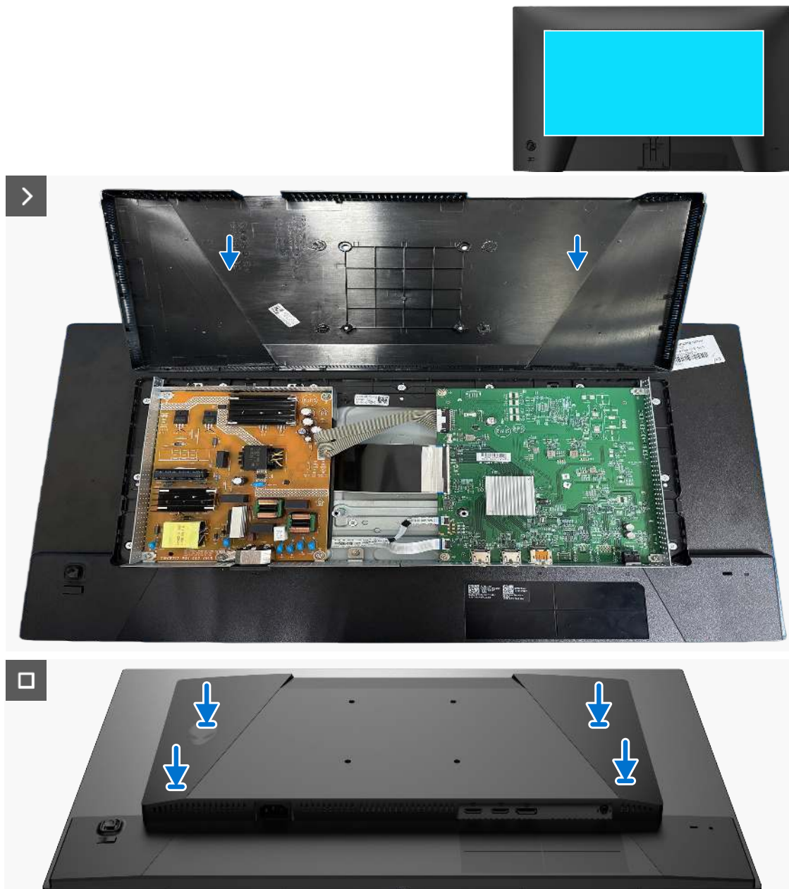
Figure 16. Installing the back cover
