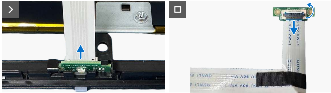
Figure 26. Removing the LED board
