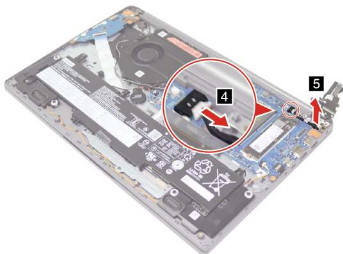
Figure 25. Disconnect and remove the DC-in cable
