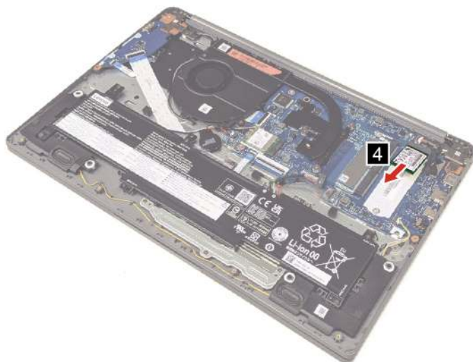
Figure 12. Remove the 2242 solid-state drive
