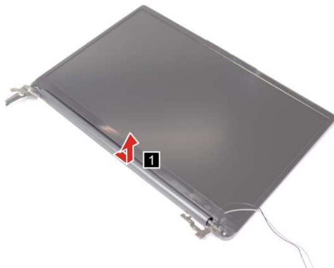
Figure 37. Remove the hinge cover
