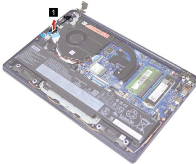
Figure 30. Disconnect cables and remove four screws
