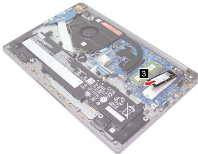
Figure 14. Remove the 2280 solid-state drive
