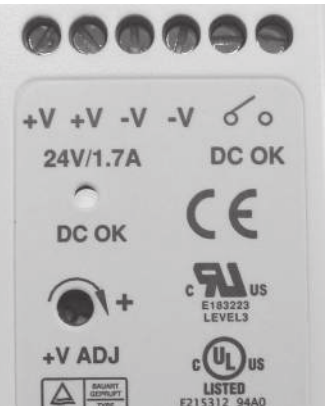
Figure 2. "DC OK" LED of DC Single Output Industrial DIN Rail Power Supply units.
