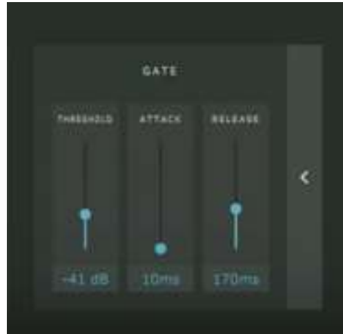
Gate with expanded controls
