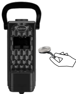
Fig. 12-B - pull out the pod holder
