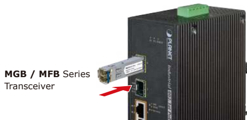
Figure 2-3: Plug-in the SFP transceiver
