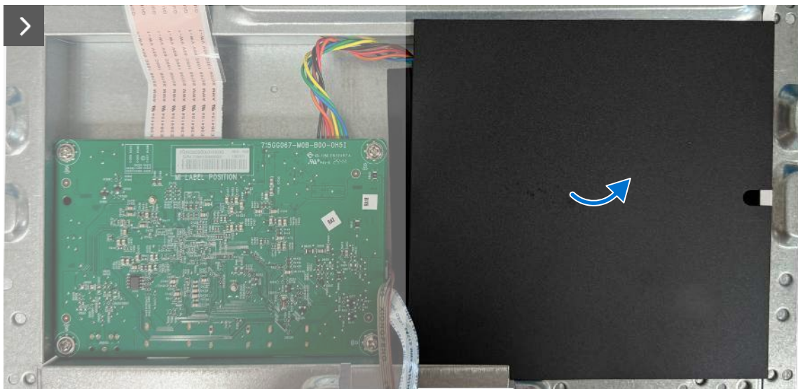
Figure 38. Removing the system board and power board (AW2726DL)
