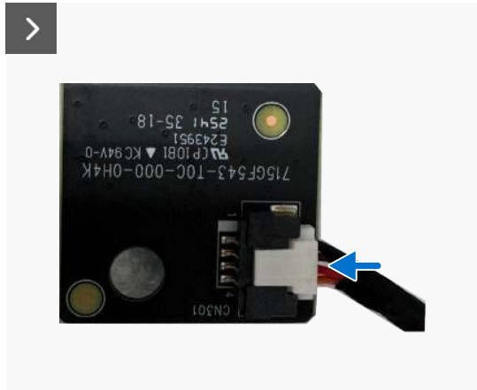
Figure 25. Installing the LED board (AW2726DL)
