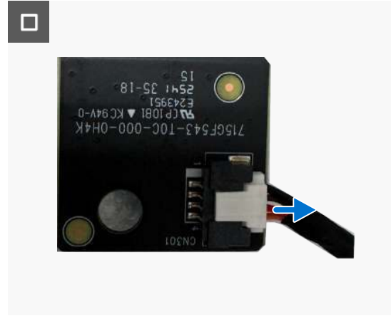
Figure 23. Removing the LED board (AW2726DL)
