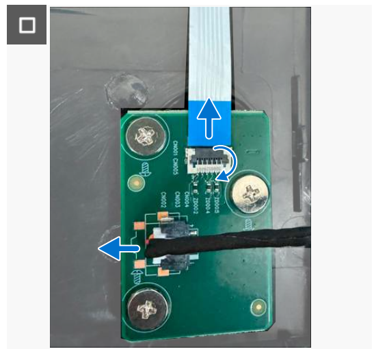
Figure 18. Removing the back cover (AW2526HL)
