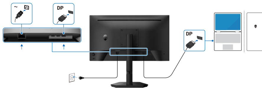
Figure 11. Connecting the DisplayPort cable
