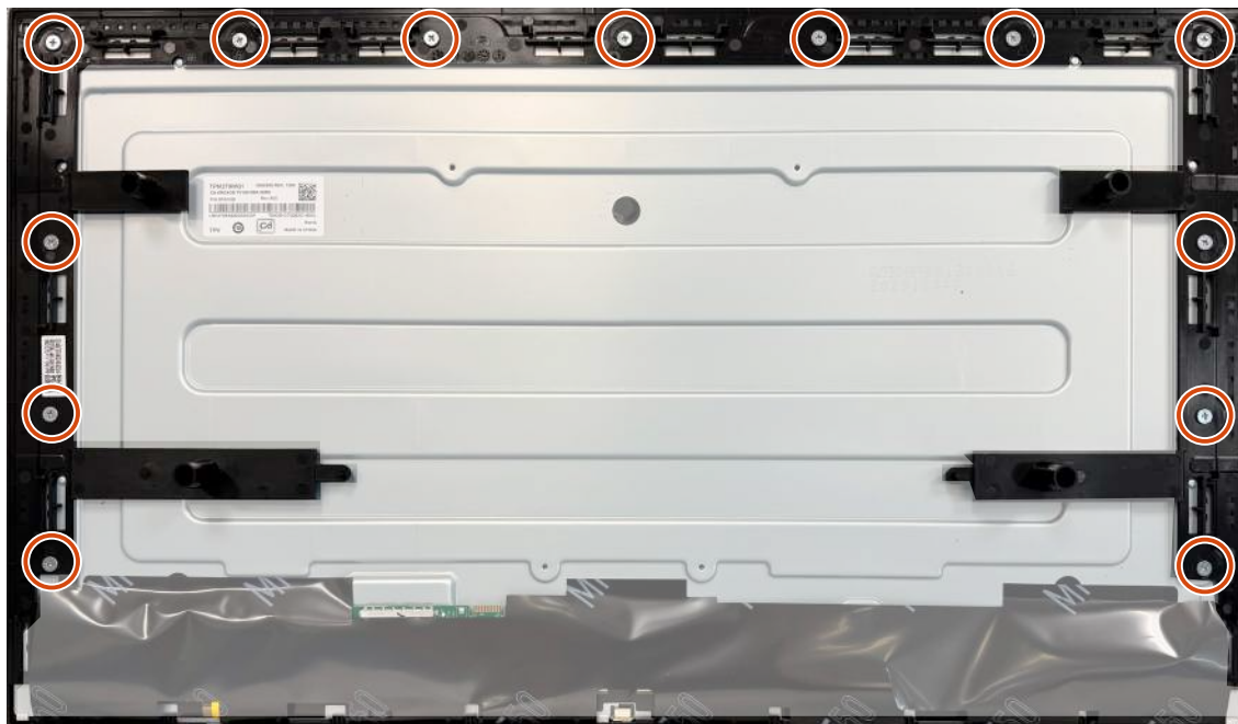
Figure 47. Installing the middle frame (AW2726DL)
