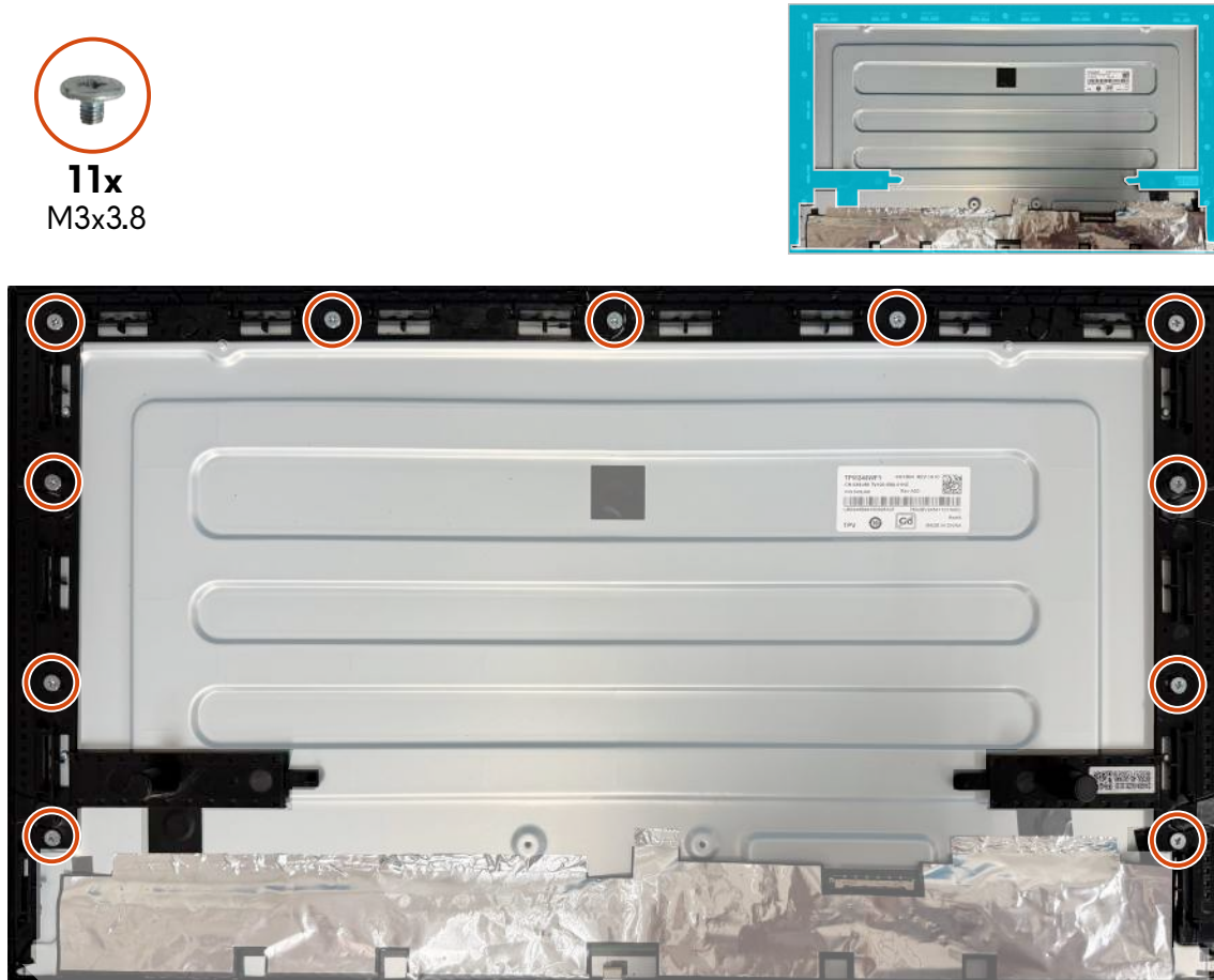
Figure 46. Installing the middle frame (AW2526HL)
