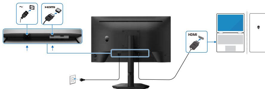
Figure 12. Connecting the HDMI cable
