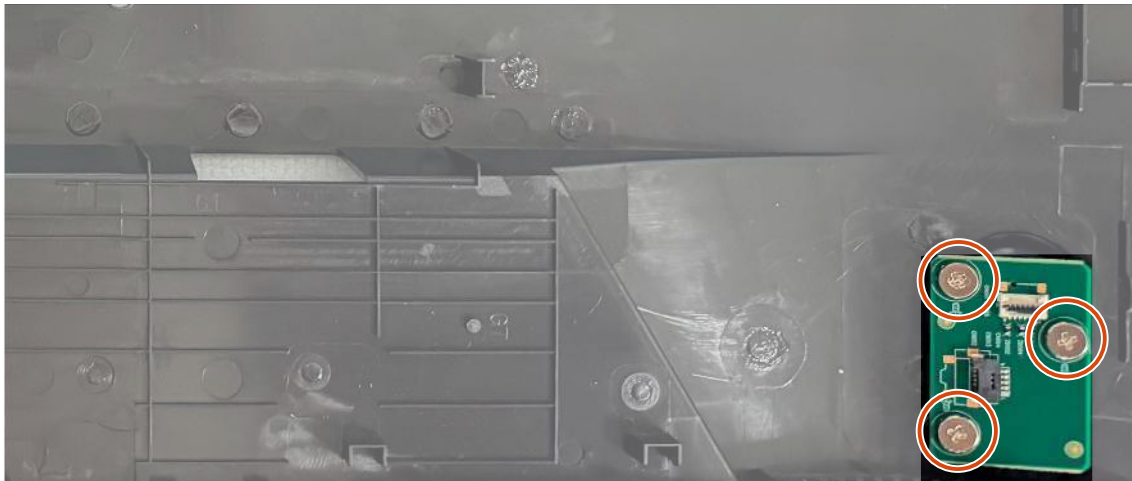
Figure 26. Removing the keypad board
