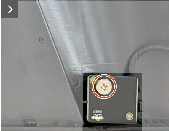
Figure 23. Removing the LED board (AW2726DL)
