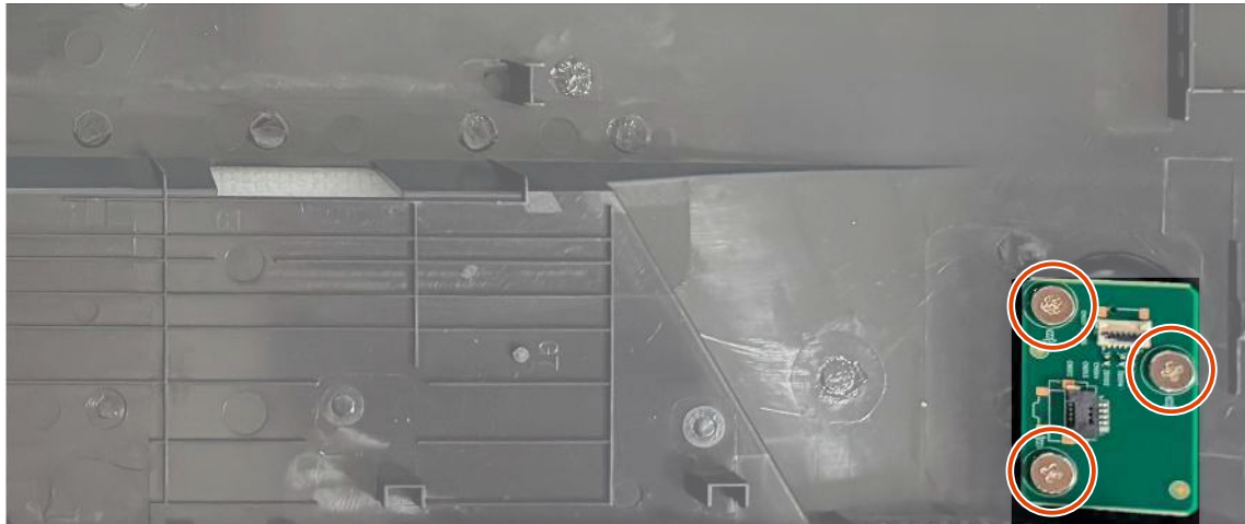
Figure 27. Installing the keypad board
