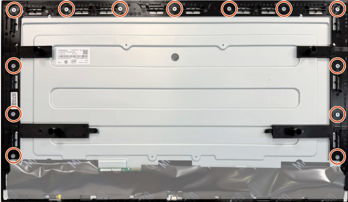
Figure 45. Removing the middle frame (AW2726DL)
