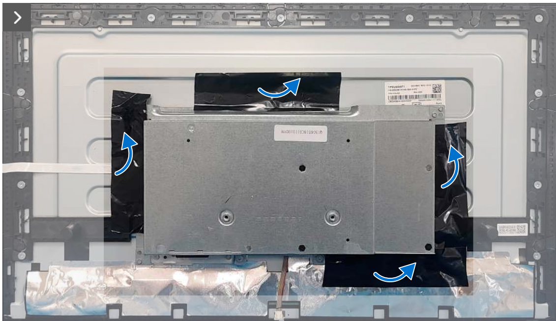
Figure 28. Removing the metal shield (AW2526HL)
