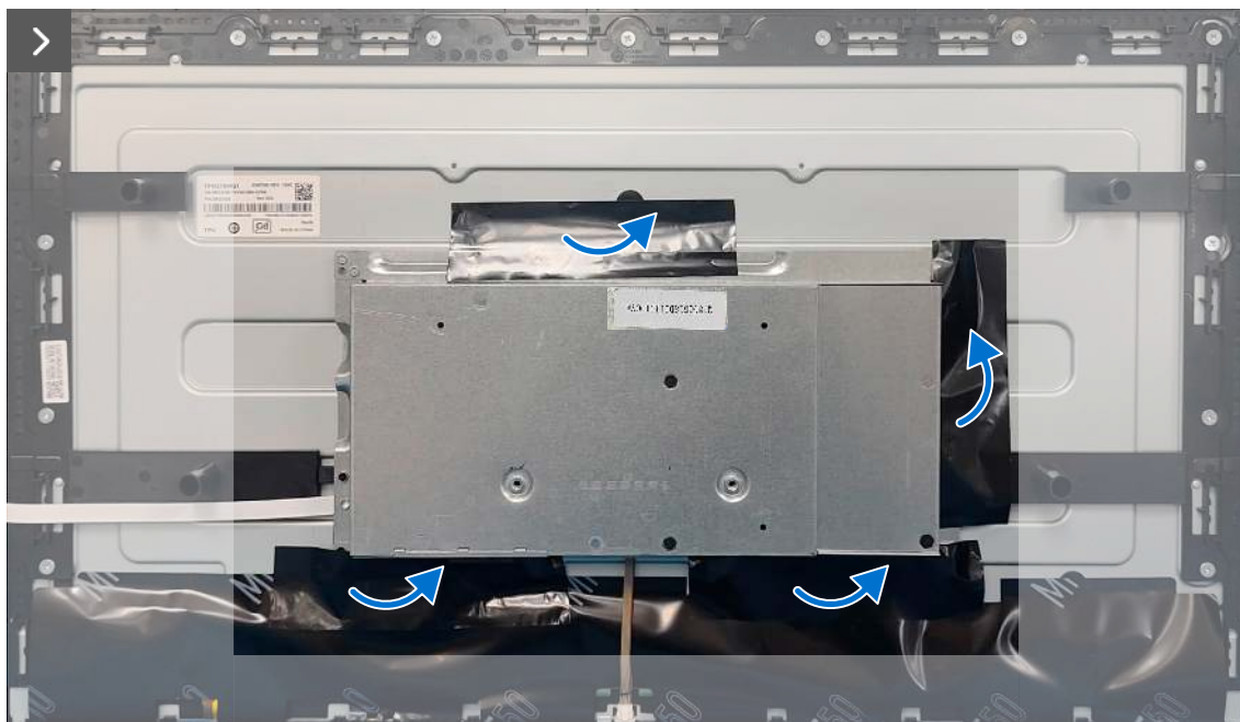
Figure 30. Removing the metal shield (AW2726DL)
