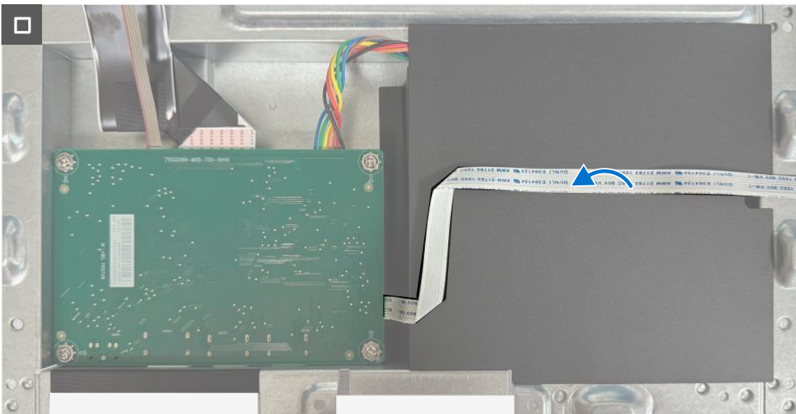
Figure 41. Installing the system board and power board (AW2526HL)
