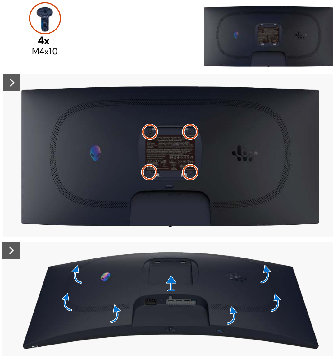
Figure 17. Removing the back cover
