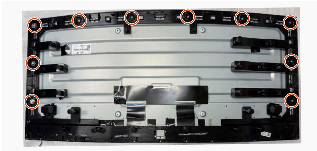
Figure 34. Installing the middle frame
