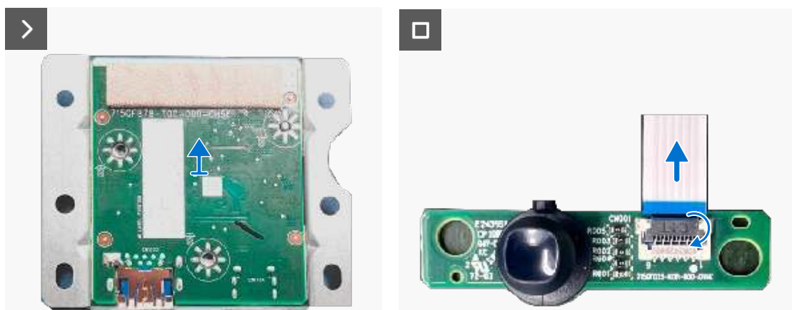
Figure 22. Removing the I/O board and joystick-button board
