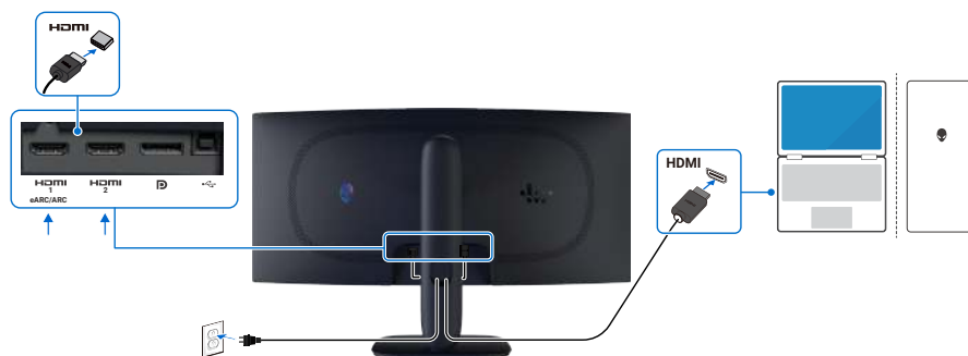
Figure 10. Connecting the HDMI cable
