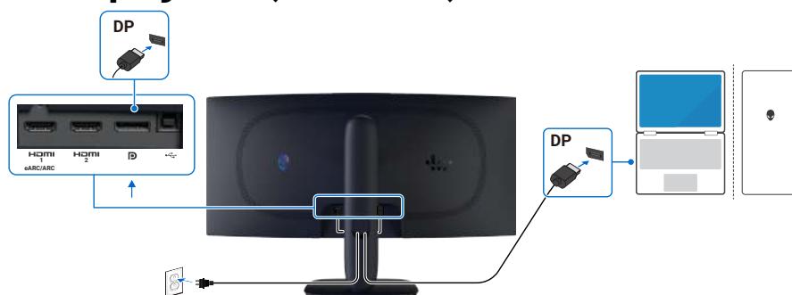
Figure 9. Connecting the DisplayPort (DP to DP) cable
