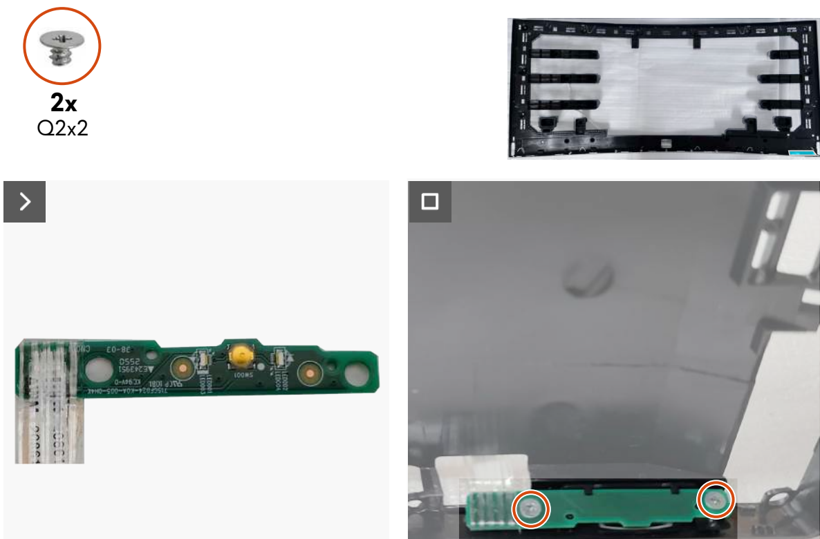
Figure 38. Installing the power-button board
