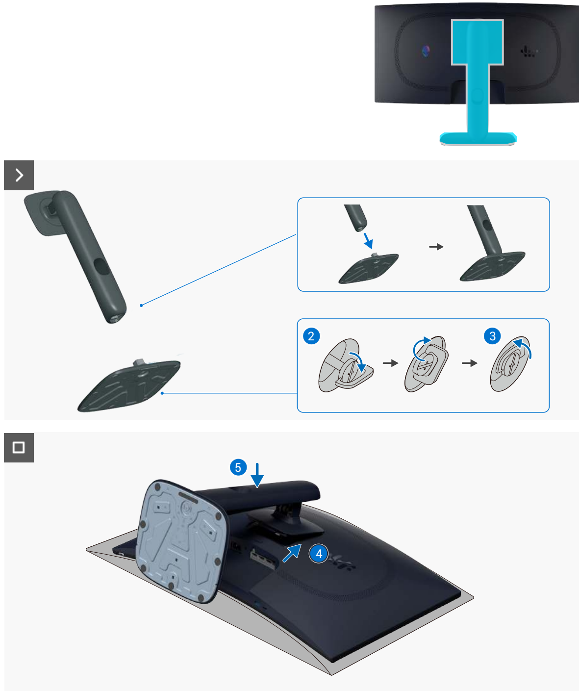
Figure 15. Installing the stand
