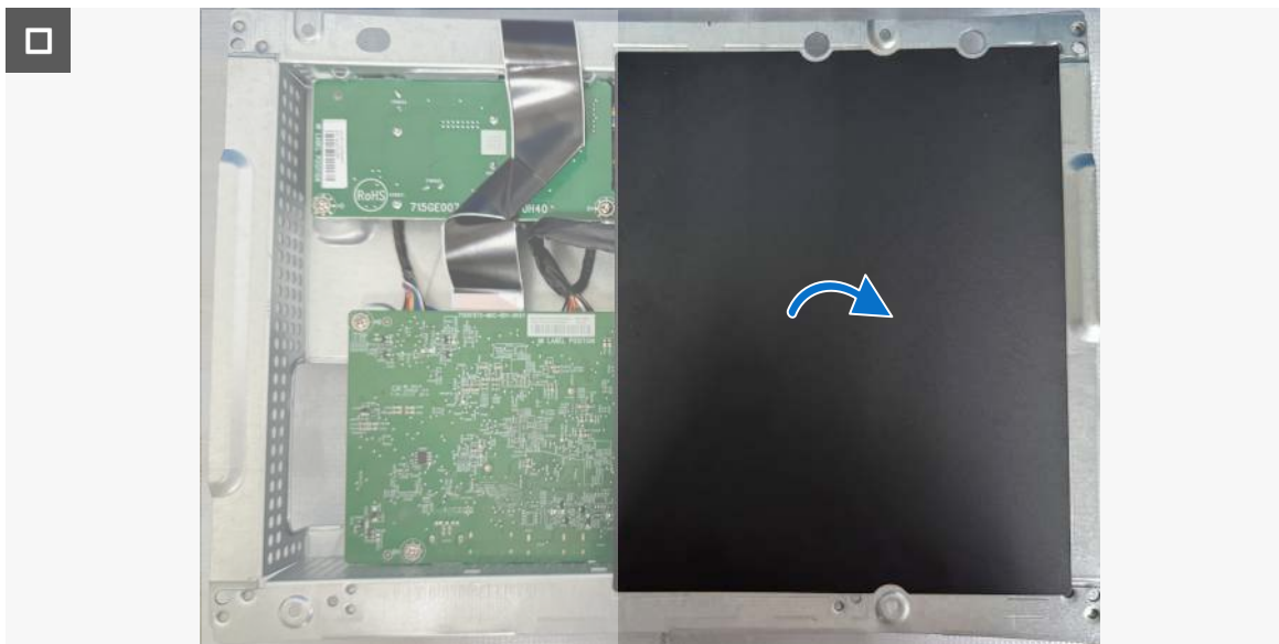
Figure 32. Installing the system board, power board and converter board
