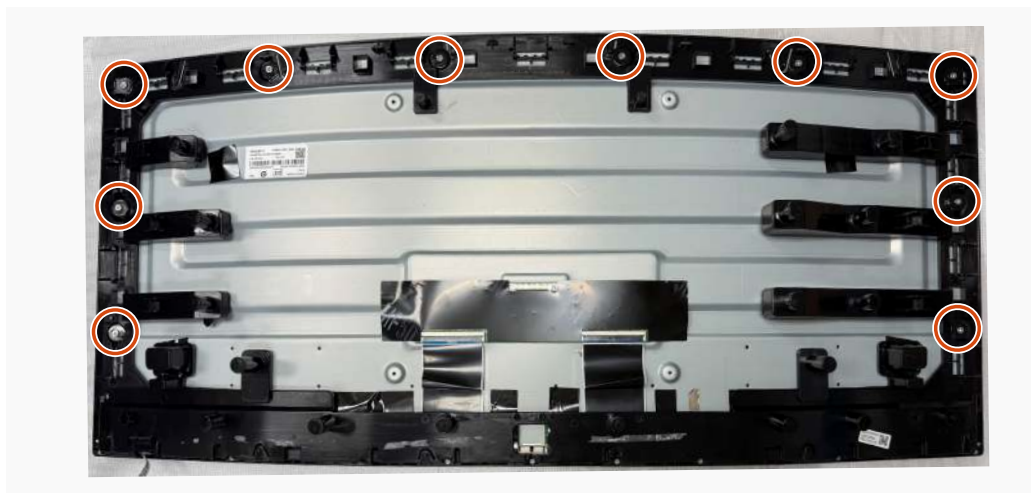
Figure 33. Removing the middle frame
