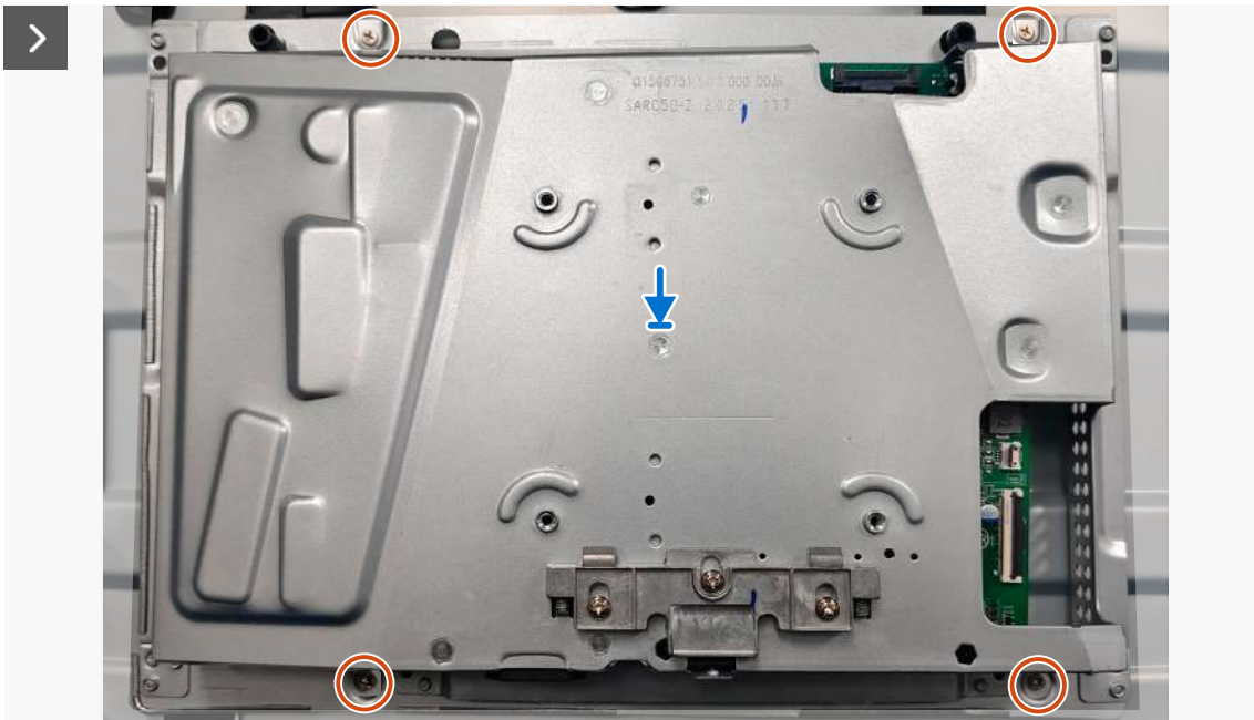
Figure 28. Installing the metal shield
