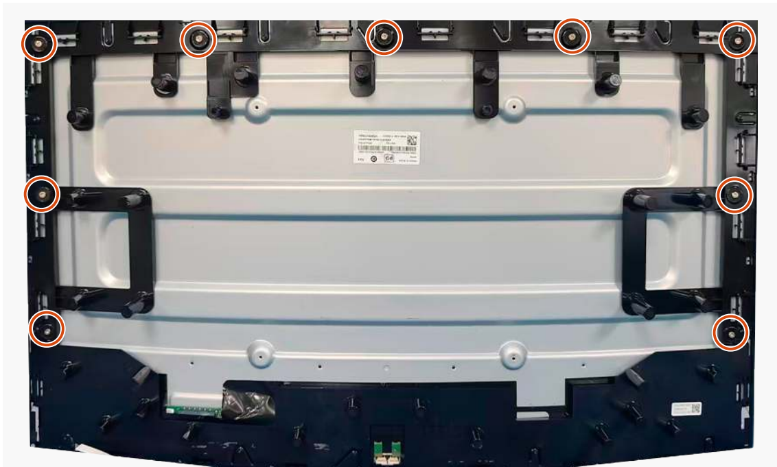
Figure 36. Installing the middle frame
