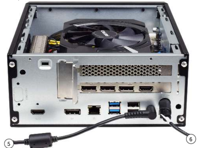
XH510G2 with two power adapters connected Graphics card: MSI GeForce RTX 3060 AERO ITX 12G OC
