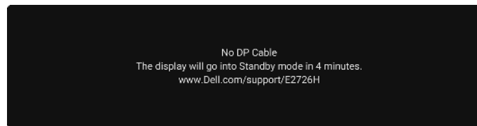
Figure 21. DP cable disconnected warning message
