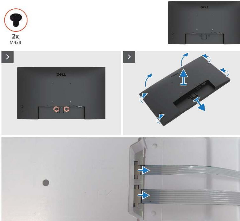
Figure 11. Removing the back cover
