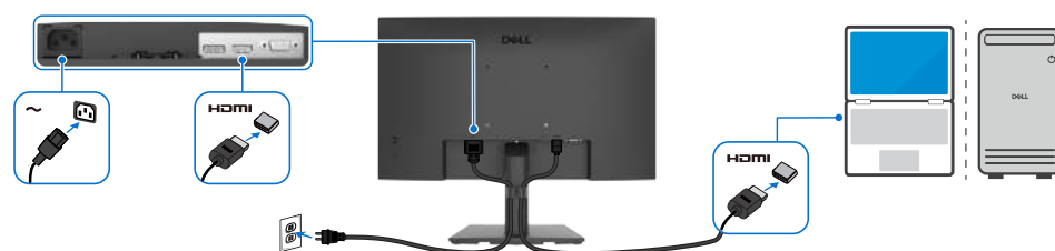
Figure 8. Connecting the HDMI cable
