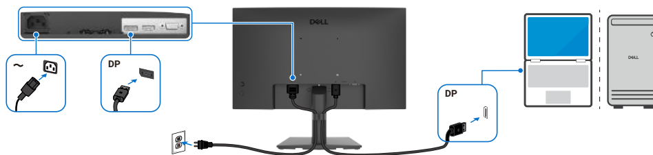
Figure 7. Connecting the DP cable
