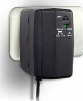
UPS in operation
