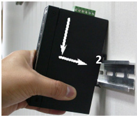
Figure 5: Install Industrial Equipment in DIN-Rail mount.
