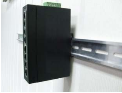
Figure 6: Industrial Equipment installed in DIN-Rail mount.
