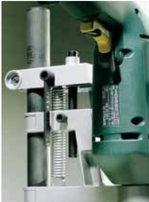
depth of cut set by depth stop
