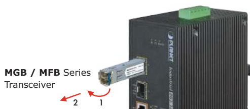
Figure 2-4: Pulling out from the transceiver
