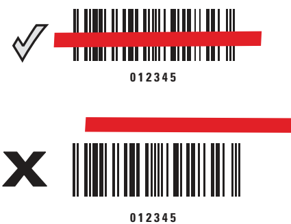
Figure 2-6 Scanning Orientation with Aiming Line
