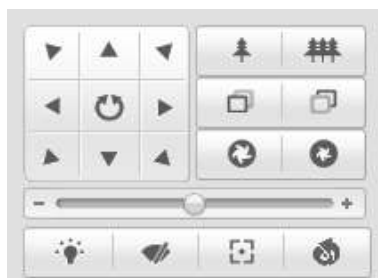
Figure 5-3 PTZ Control Panel
