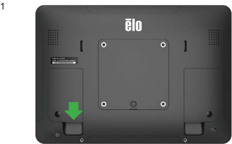
Remove the left side cable cover by lifting upward
