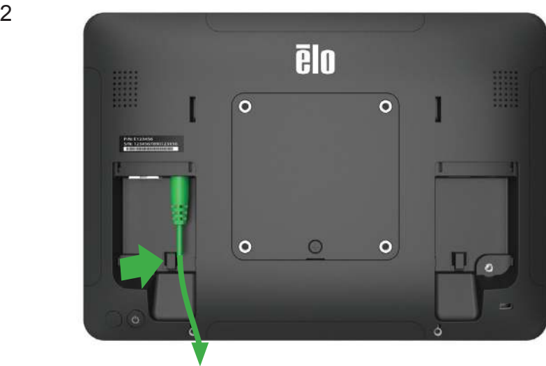
Connect the power cable. The system will power on automatically when plugged in. A tie-wrap can be used to secure the power cable from accidental removal.
