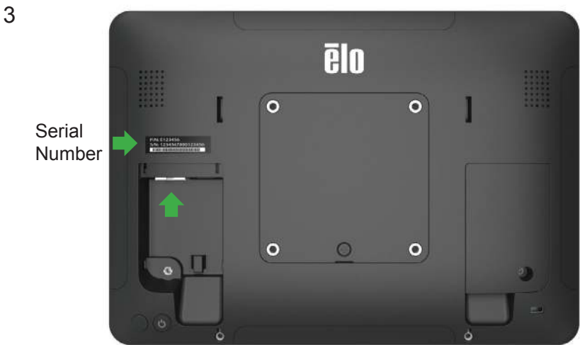
The system must be connected to a network for software setup. Connect an Ethernet cable now or setup WiFi in step 5. Note the device serial number for use in step 6.
