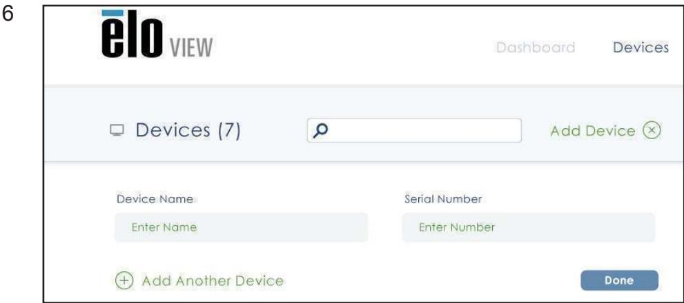
To add your device to your EloView account, go to the EloView web portal at manage.eloview.com . After logging in, go to the 'Devices' page, then click the 'add device' button. Enter the device serial number and a name for the device. Click 'done'. Your device is now linked to your EloView account and will play the assigned content in safe kiosk mode. You can also pre-set your devices in your account. Visit www.eloview.com for details.
