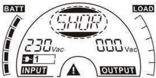
■ Figure 6.5 The Fault mode
