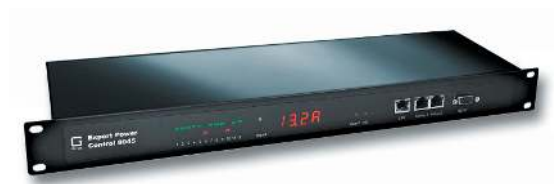
Expert Power Control 8045-2: 12 IEC-Lock outlets on the rear panel prevent unintentional disconnection of the cables
