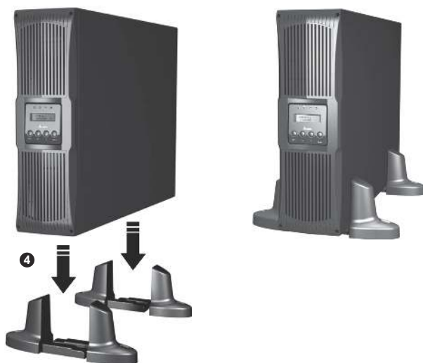
(Figure 4-6 : Place the UPS Inside the Tower Stands)
