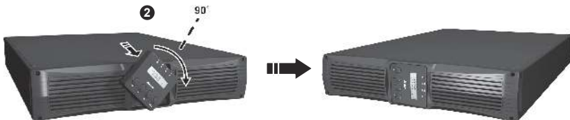
(Figure 4-4 : Rotate the UPS Control Panel)
