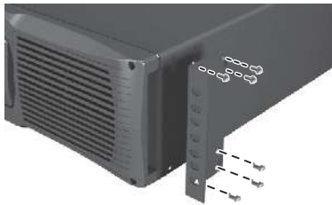
(Figure 4-1 : UPS Bracket Ear Installation)
