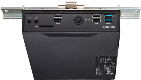
Sample photo: Shuttle XPC slim DS10U mounted on a 35 mm DIN-Rail.
