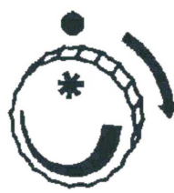
Setting of the required room temperature (max. 15°C)
