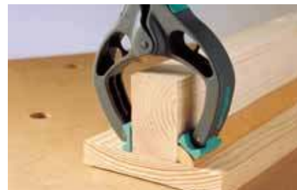
movable clamping jaws adjust to the workpiece
