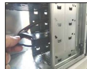
Sliding the Mounting Bracket into the 3.5" Hard Drive Slot
