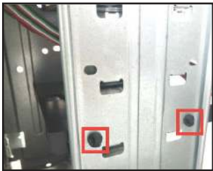
Inserting the Plastic Pegs into the Computer Chassis
