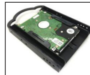
Inserting a Hard Drive into the Mounting Bracket
