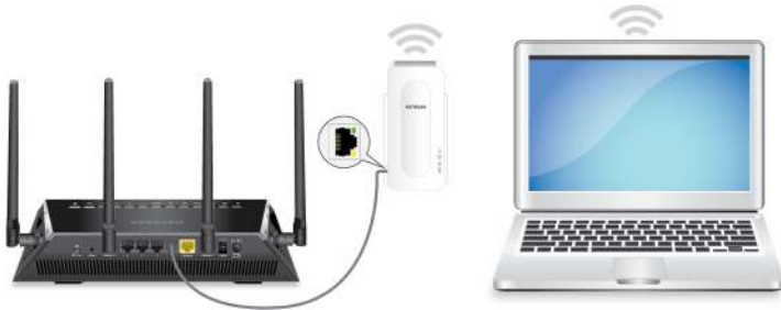
Figure 4. Extender in access point mode
