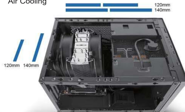
CPU cooler blowing downwards 3.5" HDD x 2, 2.5" SSD x 3
