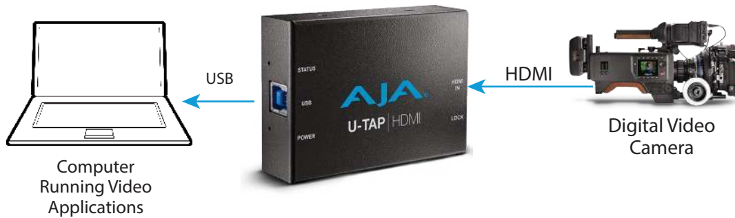
Figure 5. Typical U-TAP-HDMI Laptop System Connections
