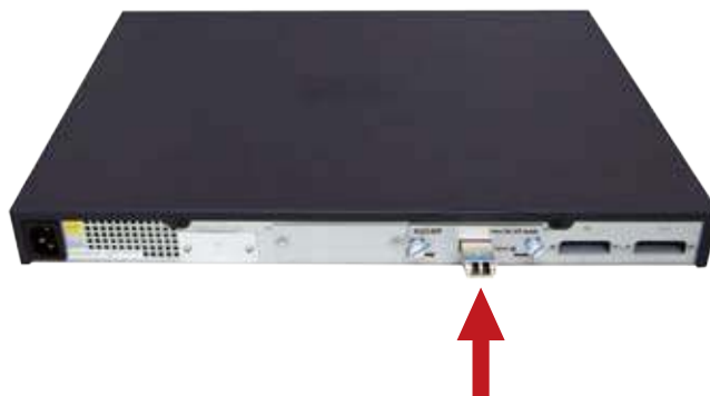
MTB 10GBase-LR/SR Module in the 10G XFP slot
