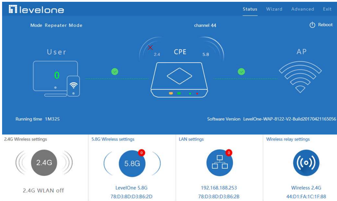
P27 WAP-8021 Status in Repeater Mode
