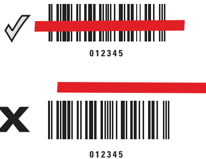
Figure 2-3 Scanning Orientation with Aiming Line
