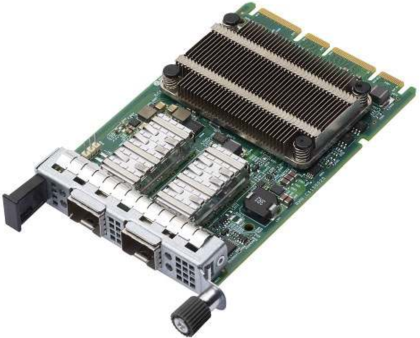
Figure 1: BCM957414N4140C OCP 3.0 SFF Network Adapter
