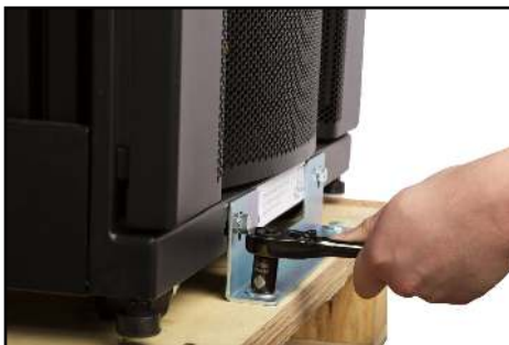
Removing the Bolts
