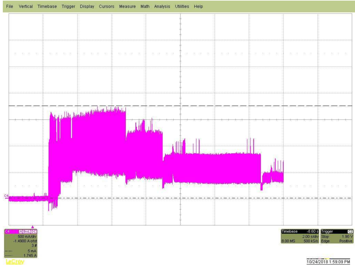
Figure 1. Typical 12V startup and operation current profile
