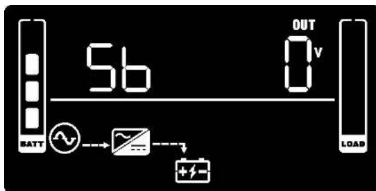
Figure 18: Display in standby mode
