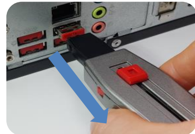
③ Pull straight out to remove a Port Lock
