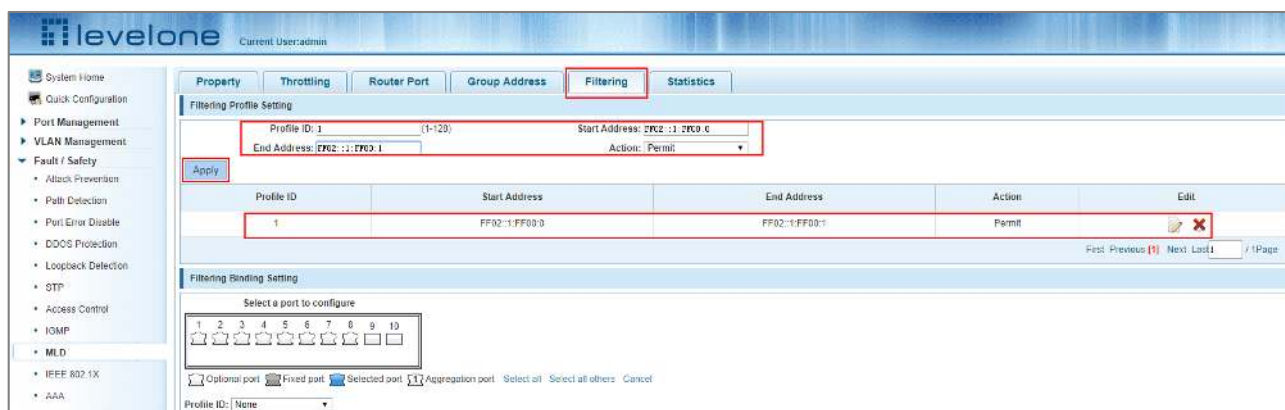
Figure 6-58: Configuring MLD Filtering
