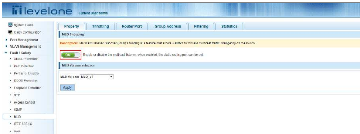
Figure 6-53: Disabling the Multicast Listener Function
