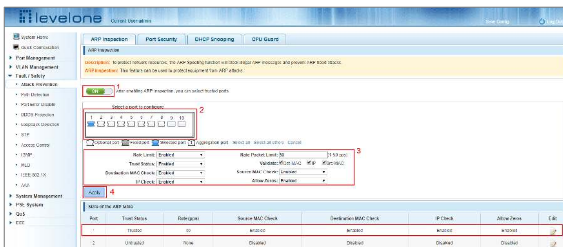
Figure 6-2: Configuring ARP Inspection
