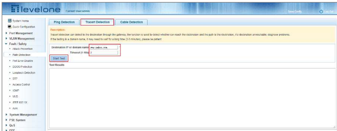
Figure 6-18: Trace Route Test
