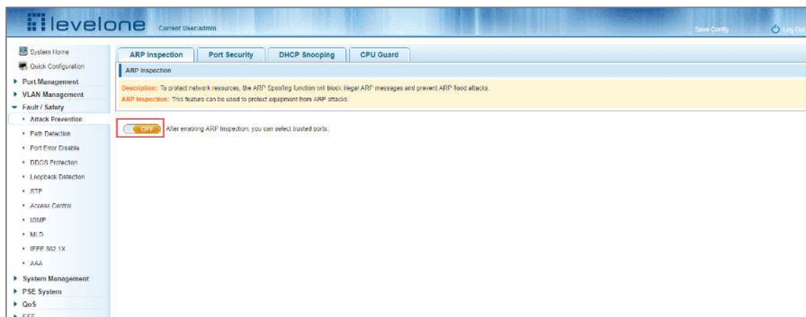
Figure 6-1: Showing the Port ARP Inspection configuration
