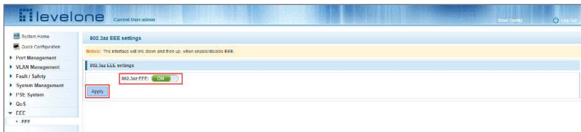
Figure 10-2: Enabling 802.3az EEE
